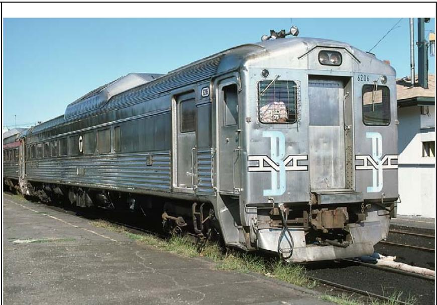
Former B&M 6206 in 1977 at Rockport, MA, USA – sold to MBTA in 1976 but still retaining B&M lettering in photo. Built in 1955 by the Budd Company and rebuilt in 1982 by Morrison-Knudson as a cab-control car lettered MBTA #1404. It is now lettered VTRX 106 and is used on the Guelph Junction Express tourist train. Photo by George W. Hamlin and used with permission.
